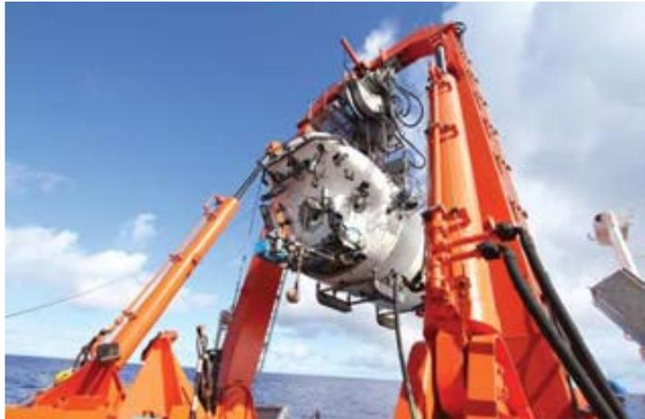
The hydraulically operated A-Frame lifted the submersible above water before it was lowered, and successfully lifted it back onto the Mother Ship, Xiangyanghong9. In addition to the launch and recovery winches, Caley supplied two bespoke winches to handle scientific instruments for ocean bed research.
